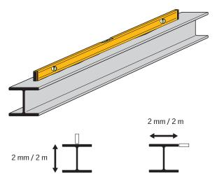
The following standard steel profiles are suited for installation of VELUX modular skylights in Wall-mounted Longlight solutions.
