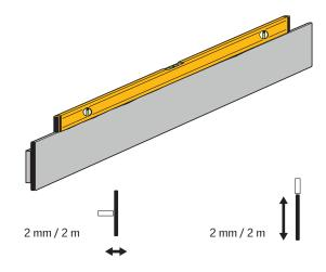
The following standard flat steel profiles are suited for installation of VELUX modular skylights in Wall-mounted Longlight solutions.
