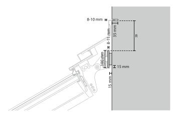
Steel, concrete or wood construction with flat steel profile
