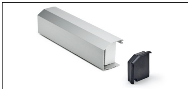
Cover caps are made of aluminium (2mm), the surface is treated either as nature anodized or polyester powder coated. Polystyrene insulation is installed inside the cover cap. EPDM rubber plugs are pushed on the cover caps in the ends.
