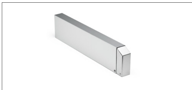
Flashings are made of aluminium (1 mm). The surface is treated either as nature anodized or polyester powder coated.
