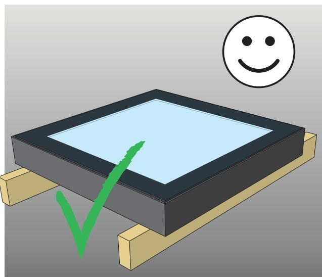
**ENGLISH: Note:** Do not place the top unit directly on a hot roof as this may damage the glazing.
