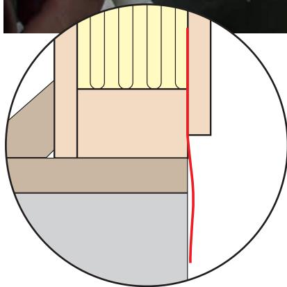
**ENGLISH:** Remove the tape from the bottom of the frame to release the vapour barrier. Allow the vapour barrier to suspend in the hole.
