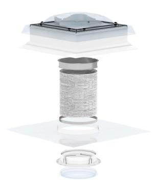
The VELUX sun tunnel for flat roof with flexible tunnel is the perfect choice for VELUX sun tunnel installations when rigid tunnels cannot be used – i.e. when there is a beam or other obstacle between the roof and the ceiling. Recommended for lengths between 0.4 m and 1.5 m for pitched roofs and 0.2 m and 0.9 m for flat roofs.
