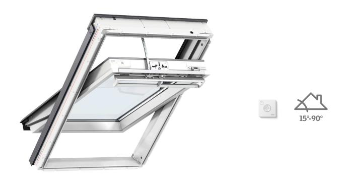
The VELUX electric, centre-pivot roof window GGU is a wired solution that operates remotely using a wall switch – perfect for both in- and out-of-reach installations. The roof window has an integrated motor and a rain sensor that automatically closes the window if it rains. Moisture-resistance makes it ideal for kitchens and bathrooms.
