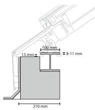
Steel, concrete or wood construction with steel profile
