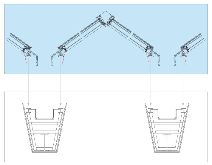
On-site sub-construction This is not delivered by VELUX Commercial
