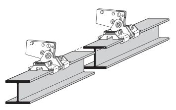
Connestion of steel profiles must not collide with clamps
