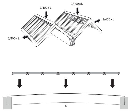
A: Beams can be constructed with a camber height to withstand the weight from the modules
