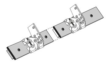
· Connection of flat steel profiles must not collide with clamps
