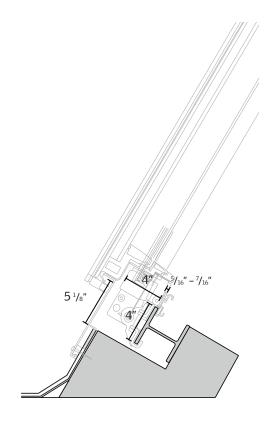
Concrete construction with steel profile
