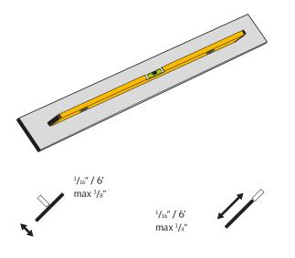
Steel or wood construction with flat steel
