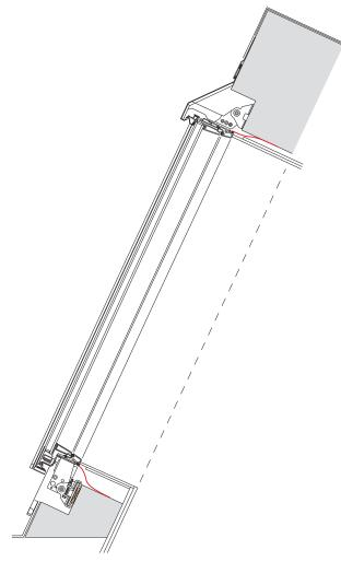
Steel or wood construction with flat steel
