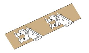
The sub-construction can be finished at the top with steel profile or flat steel profile, which provides a level and stable surface for the skylight modules and forms a base for fitting mounting brackets with clamps.
