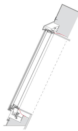
Steel or wood construction with steel profile
