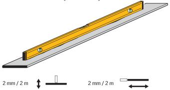
The following standard flat steel profiles are suited for installation of VELUX modular skylights in Step Longlight solutions.
